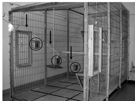
Figure 4. Photograph of the social behavior enclosure taken in front of the clear lexan side to display the food delivery tubes (arrows) and food bins (circled) attached to the left side of the cage for delivering food pellets during the food competition condition.
