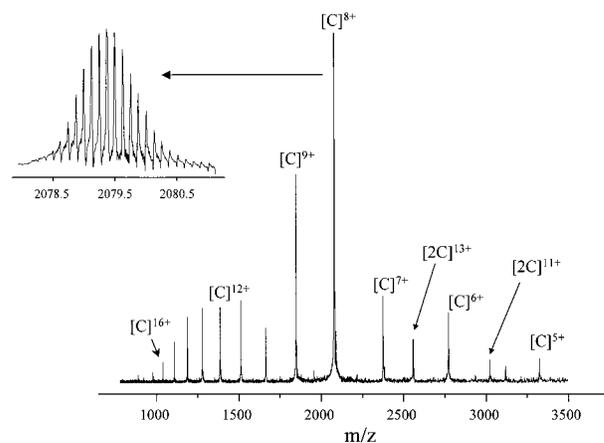
FIGURE 1: ESI–FTICR mass spectrum of calmodulin in ammonium acetate buffer, 5 mM, pH 5.9. Inset shows the isotopically resolved pattern of the 8<sup>+</sup> charge-state.
