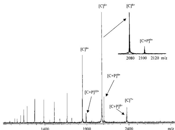
FIGURE 3: ESI-FTICR mass spectrum of calmodulin with RS20 peptide (concentration ratio 1:1.5) in ammonium acetate buffer, 5 mM, pH 5.9, in the absence of calcium. Inset shows the expansion of the  $8^+$  calmodulin charge-state. P represents RS20.
