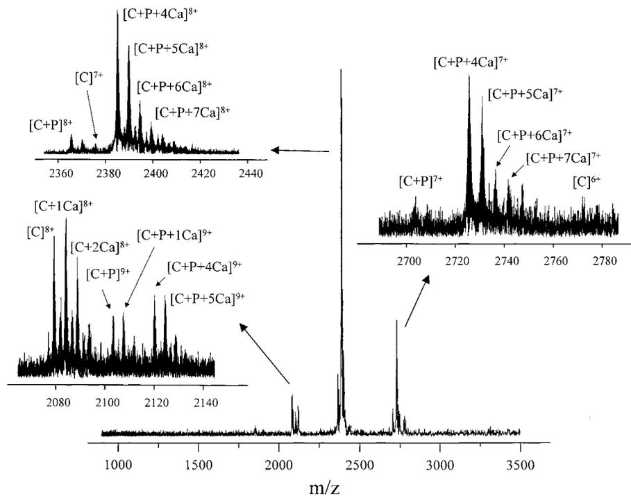
FIGURE 5: ESI–FTICR mass spectrum of calmodulin with RS20 peptide (concentration ratio 1:1.5) in ammonium acetate buffer, 5 mM, pH 5.9, containing 0.1 mM  $\text{CaCl}_2$ . Insets show the expansion of the lower charge-states. P represents RS20.
