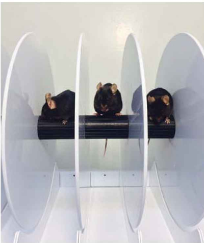
Figure 13–51 The rotarod assay for testing motor coordination. At the beginning of the experiment, mice are placed on a stationary rod; the separate compartments shown in the photograph allow simultaneous testing of multiple animals. The rod is connected to a motor with an adjustable speed. Typical experiments include running the motor at a constant speed (for example, 10 revolutions per minute, or rpm) or a speed that increases (for example, from 5 to 30 rpm), and measuring the period of time each mouse remains on the rod. In addition to testing motor coordination, the rotarod can also test motor skill learning (see Figure 8–18D). (Courtesy of Mehrdad Shamloo.)
